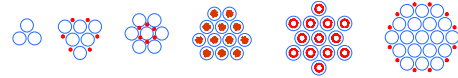
FIG. 4. (Color online) The collection of bundles used for model calculations. Bundles of 3, 6, 7, 12, 13, 18, and 19 tubes. The sixth bundle is shown in Fig. 5. The different sites occupied by Rb + ions are shown in the figure. From left to right: raw, grooves (GS), triangular channels (t), interior (i) random, interior (i) surface, and grooves (GS).
